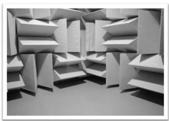
The semi-anechoic chamber then forms a controlled environment with the surrounding acoustic conditions behaving as a sterile version of the real world. In this way accurate measurements of the sound inside and outside the vehicle can be made under operating conditions.
